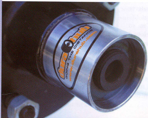
The new oil-based Durahub bearing protector.
