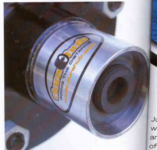
A shot of the completed installation. Note the sight lens which allows trailer owners the ability to check oil levels easily.
